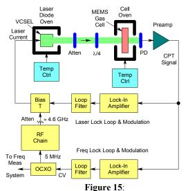
Testbed configuration for closed-loop operation
