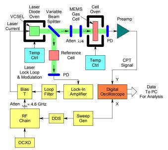
Figure 4: Testbed configured for CPT spectroscopy
