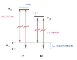
Figure 6: Cesium D1 and D2 CPT resonance levels
