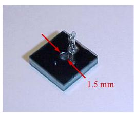
Figure 13: Prototype silicon-glass MEMS cell
