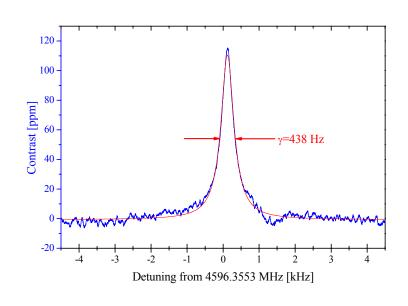
Figure 14: Relatively narrow CPT resonance in MEMS cell
