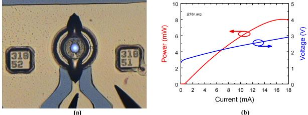
Figure 7: Prototype VCSEL device (a) photograph and (b) light-current-voltage data
