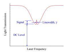
Figure 3: CPT resonance features
